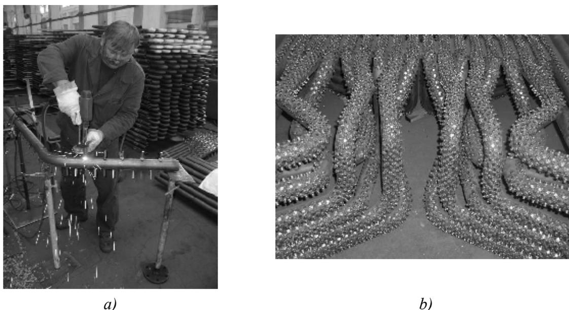
**Fig. 1** Arc stud welding on membrane panels in steam boiler production (a), detail of welded studs from boiler production (b) [7]
