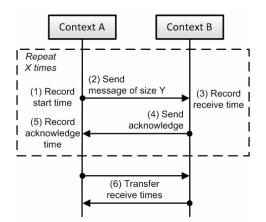
Figure 2. Evaluation scenario sequence diagram
