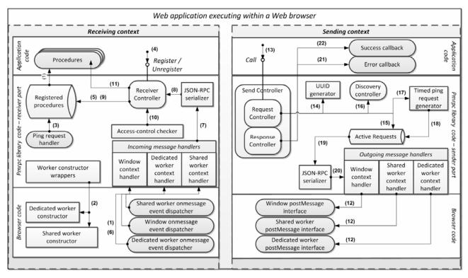
Figure 1. Architecture of the Pmrpc cross-context communication system
