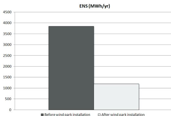
Fig. 11. ENS before and after of construction of the wind park
