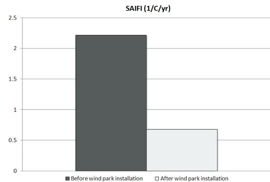
Fig. 7. SAIFI before and after of construction of the wind park
