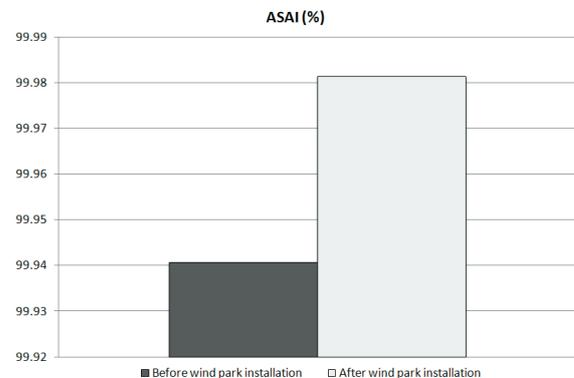
Fig. 8. ASAI before and after of construction of the wind park
