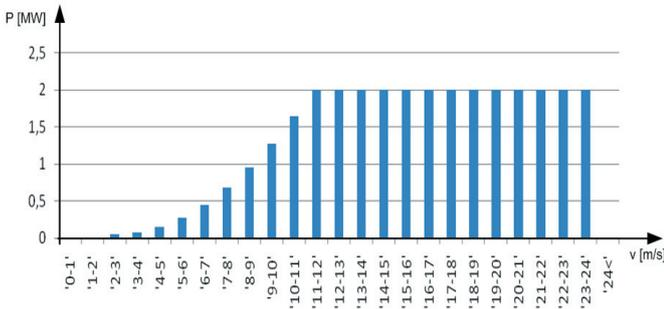
Fig. 4. Output characteristic of 2 MW WT
