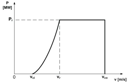
Fig. 2. Wind turbine output characteristic
