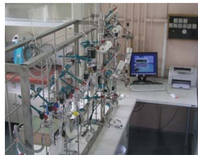
Vacuum line for preparation of graphite for ^{14}\text{C} AMS measurement technique
