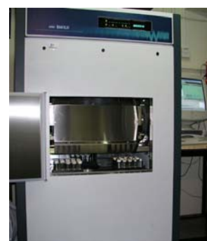
Liquid scintillation counter (LSC) Quantulus 1220 for ^{14}\text{C} and ^3\text{H} activity measurements
