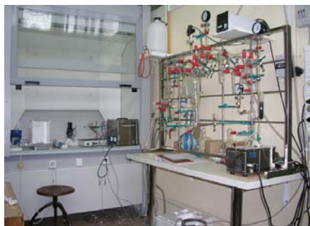
Vacuum line for benzene preparation for ^{14}\text{C} activity measurements by LSC
