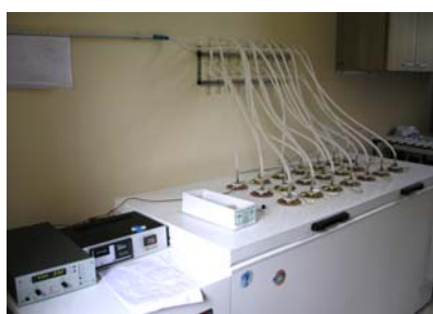
System for electrolytic enrichment of ^3\text{H} in water for ^3\text{H} activity measurement by LSC
