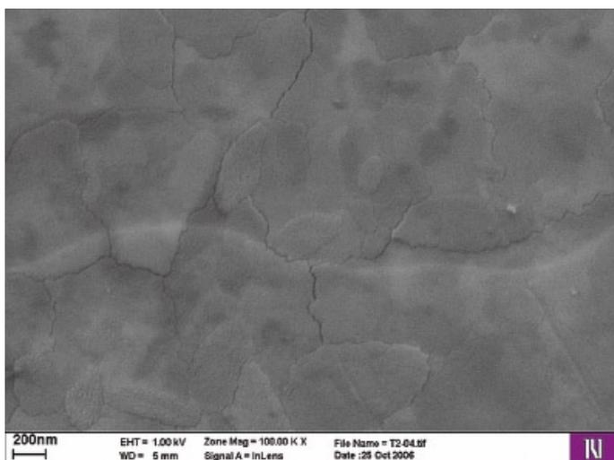
Fig. 1: SEM photograph  $\text{Fe}_2\text{O}_3$ : Li (1%), with magnification of 100.00 K.
