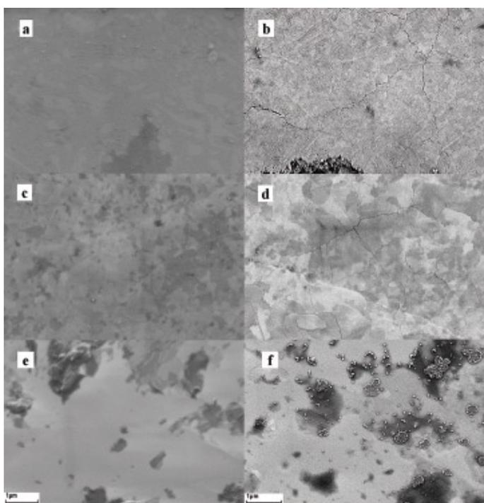
Fig. 3: SEM photographs Li free  $\text{Fe}_2\text{O}_3$  (a),  $\text{Fe}_2\text{O}_3$  with 1% (c) and  $\text{Fe}_2\text{O}_3$  with 10% of Li (e), and the same films after 8 months (b), (d), and (f), respectively.
