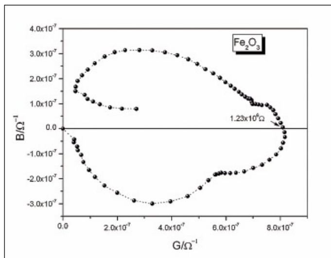
Fig. 2: (a) Admittance spectra  $\text{Fe}_2\text{O}_3$  thin film measured at room temperature and (b) equivalent circuits and schematic admittance plot for Zn electrodes.
