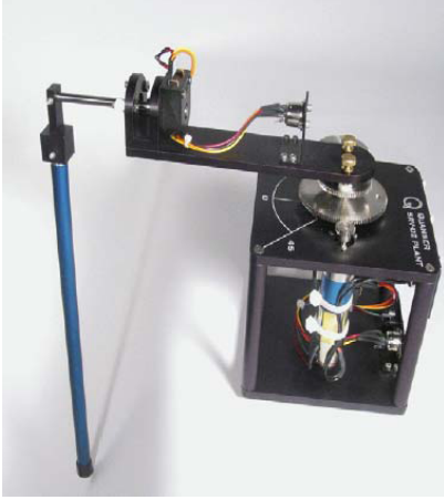
Fig. 2. Rotary pendulum gantry (RPG) laboratory model
