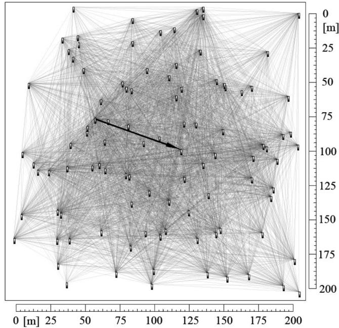
Figure 3 Simulation results for one packet transmission using flood routing algorithm. All network devices (small rectangles), packet transmission paths (thin lines) are shown, as well as the path connecting origin of the event report packet to the final destination device (thick arrow)
