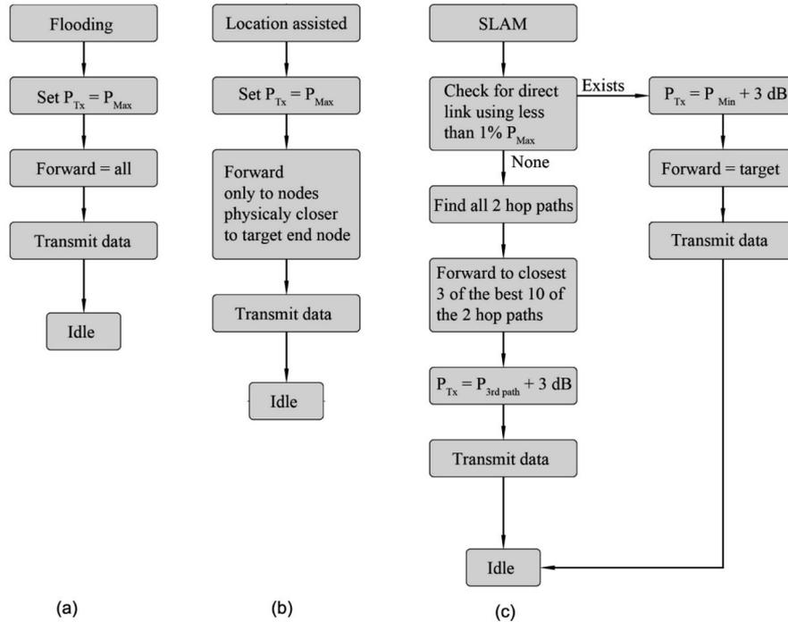
Figure 2 Smart routing sensor network diagram for the data packet transmission state showing implementation of the three routing protocols: (a) flood routing, (b) location assisted routing, and (c) SLAM routing in forward table and transmission power decisions
