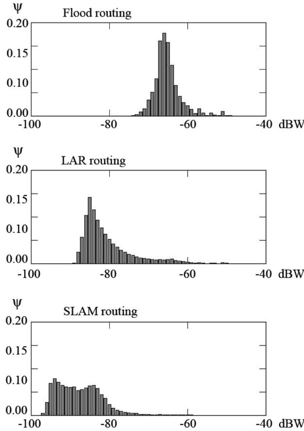
Figure 6 Interference histograms for one packet routing simulation showing probability ( $\psi$ ) of interference levels for map tiles for: flood routing (top), location aware routing (middle) and SLAM routing (bottom)
