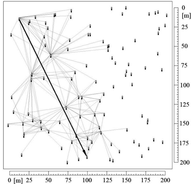
Figure 5 Simulation results for one packet transmission using SLAM routing algorithm. Shown here are all packet transmission paths (thin lines) as well as the direct path (thick arrow)
