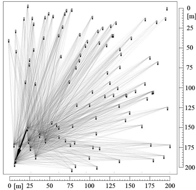
Figure 4 Simulation results for one packet transmission using location aware routing algorithm. Shown here are all packet transmission paths (thin lines) as well as the direct path (thick arrow)
