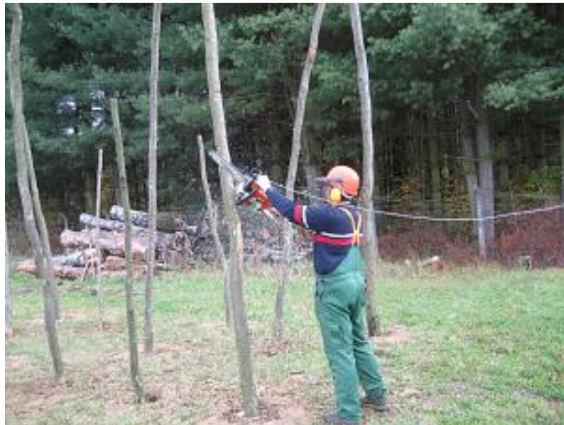
Figure 4: Vibration measurement at cutting in simulated conditions
