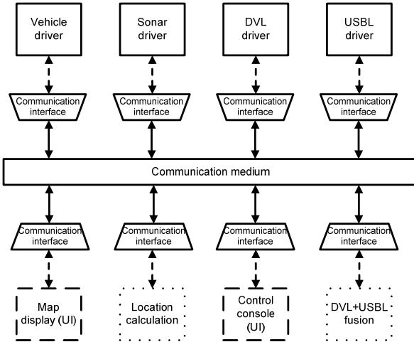
Figure 1: Architecture of system for vehicle system integration
