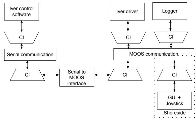
Figure 7: Iver 2 control system - logical architecture
