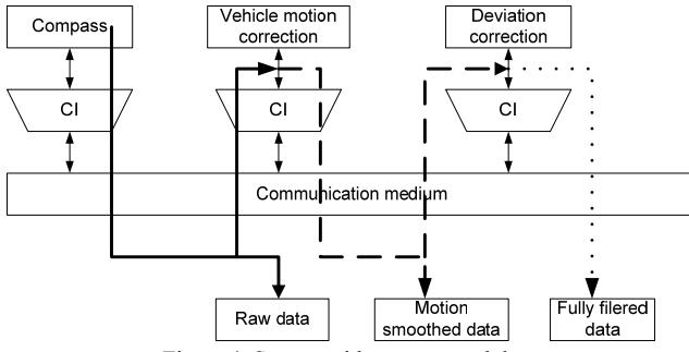
Figure 4: System with support modules
