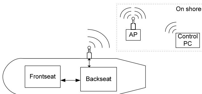
Figure 6: Iver 2 control system – hardware architecture
