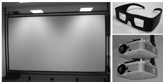
Figure 10. Parts of stereoscopic system: screen, glasses and projectors
