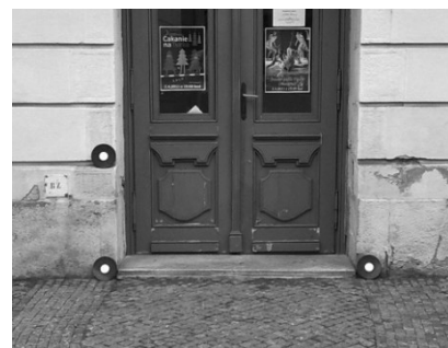
Figure 5. Markers used for scans aligning
