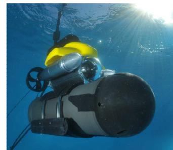
Figure 2. The UUV developed for the MCM mission.
