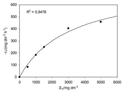
Figure 3. Influence of initial COD on substrate degradation rate for Exp. 2, (■) experimental data, and (—) model.
