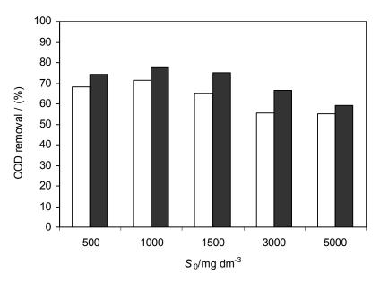
Figure 1. Efficiency of biodegradation of leachate from tobacco dust at different starting concentrations of substrate for Exp. 1 (□) and Exp. 2 (■).
