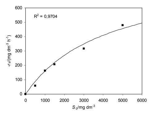
Figure 2. Influence of initial COD on substrate degradation rate for Exp. 1, (■) experimental data, and (—) model.
