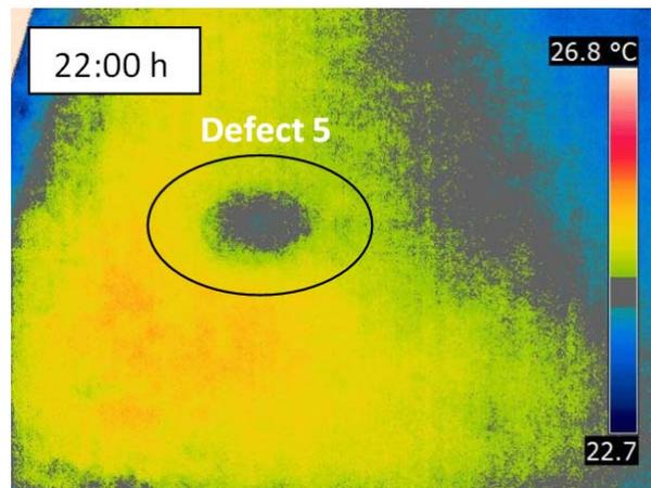
**Figure 3** Thermogram of specimen 1, defect 5, at 22.00 hours
