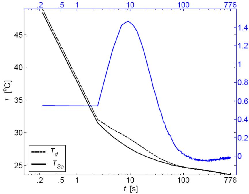
**Figure 8** Defect detection from temperature profiles [2]
