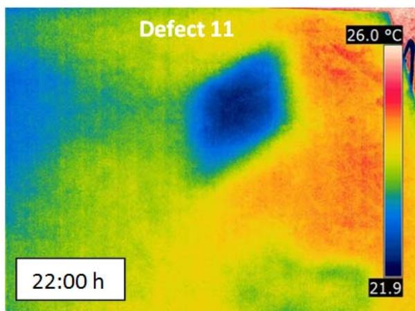
**Figure 4** Thermogram of specimen 2, defect 11, at 22.00 hours
