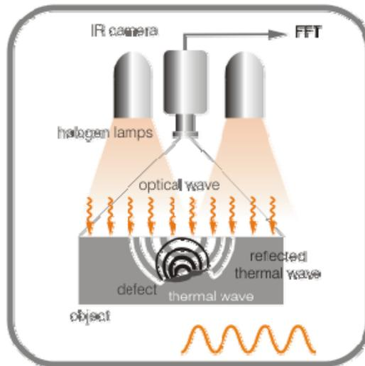
**Figure 7** Schematics of the Lock-in thermography test procedure
