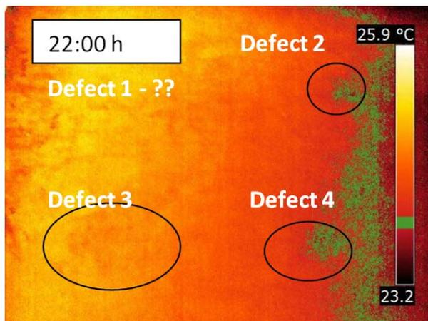
**Figure 2** Thermogram of specimen 1, defects 1 to 4, at 22.00 hours
