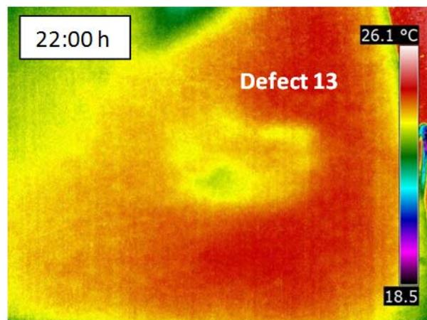
**Figure 5** Thermogram of specimen 2, defect 13, at 22.00 hours
