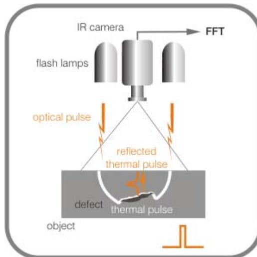
**Figure 6** Schematics of the pulse thermography test procedure
