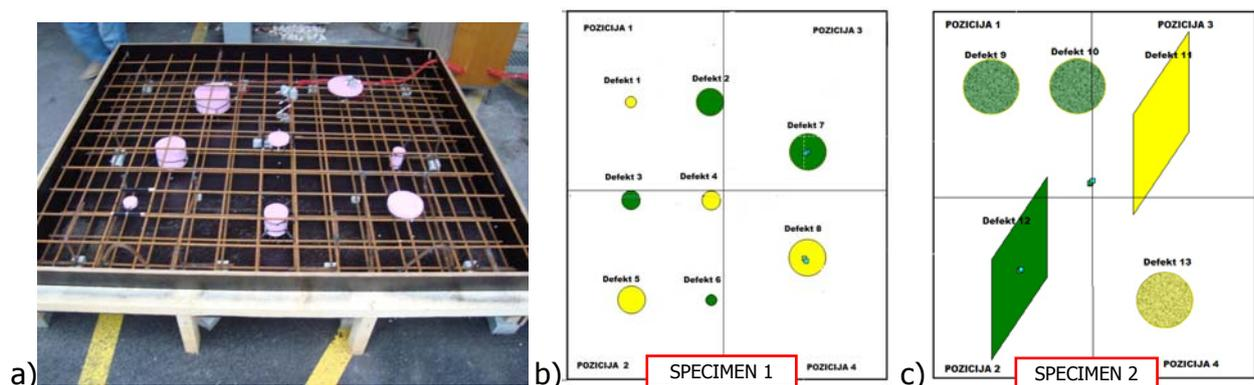
**Figure 1** Concrete test specimen including polystyrene cuboids with different sizes at different depths, a) photo before concreting, b) and c) schemes of the specimens
