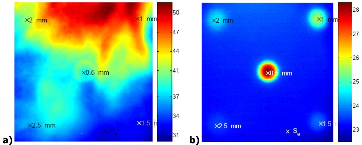
**Figure 9** Impact of non-uniform heating. Thermograms at (a)  $t=6.3$  ms; and (b)  $t=25$  ms after thermal excitation of aluminum specimen, showing defect locations [2].
