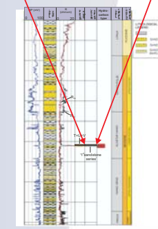
Figure 10: Schematic composite geological column (including stratigraphy, e-logs and lithology) of the well drilled typical marlstone of Lower Pontian age.
