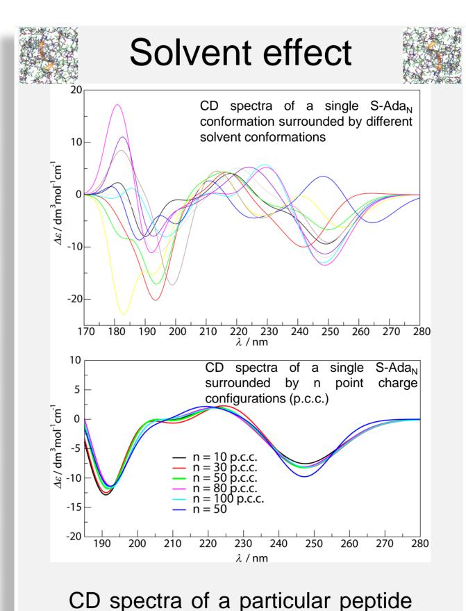
conformation greatly depends on the positions of the solvent molecules (TFE) that sorrounds it. To account for this effect in the CD calculations, we employed an average point charge field around each conformation of the peptide, which obtained superimposing coordinates of n different solvent configurations. When **n=50** p.c.c. the CD spectra of particular peptide conformation converges, as shown on the graph above.
