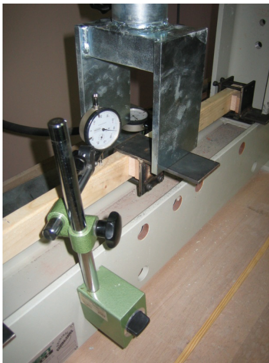
Figure 4 Measuring of deformation and applying of load
