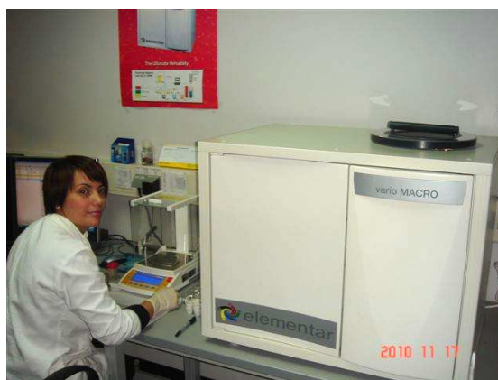
Figure 4.5.2.1 – Analysis of total nitrogen (TN %) content in dry plant tissue using the dry combustion method with the Vario Macro CHNS Analyzer.
