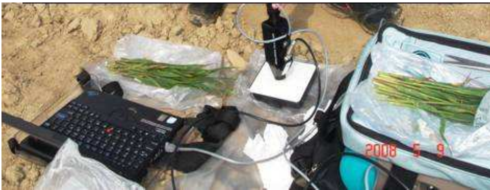
Figure 4.5.1.1.1 – Proximal reflectance measurements of winter wheat flag leaves acquired by field spectroradiometer (F8-2008).
