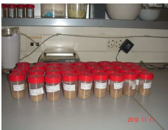
Figure 4.5.2.1.1 – Dried and grinded plant leaf and grain samples ready for the laboratory analysis.
