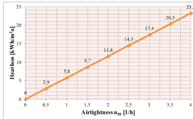
Figure 1. Heat losses regarding the airtightness of the building envelope [3]
