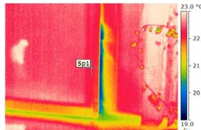
Figure 7: Poor gasket on the sliding doors
