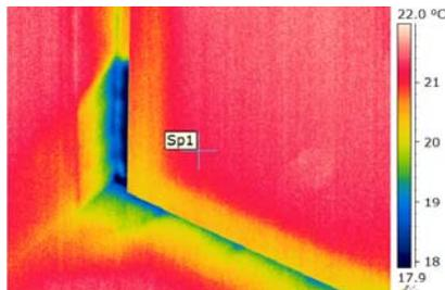
Figure 6: Poor gasket on the entrance doors
