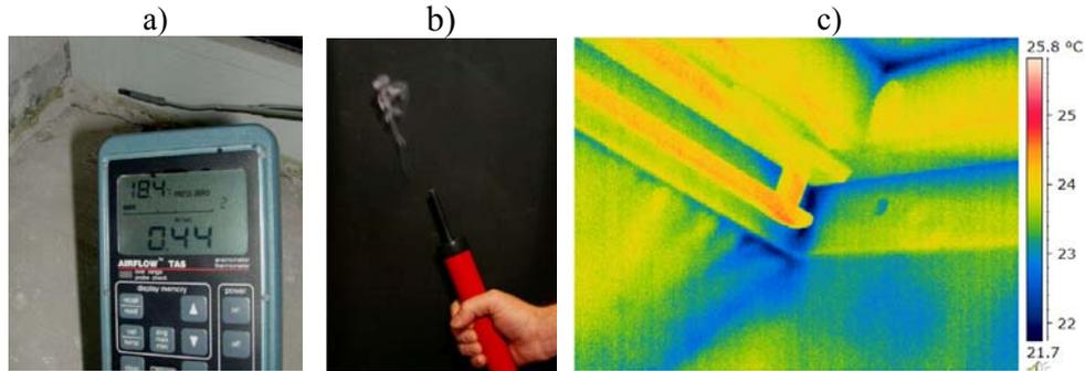
*Figure 4: Visualisation techniques of the leakages: a) air velocity meter, b) fogging, c) IR thermography*
