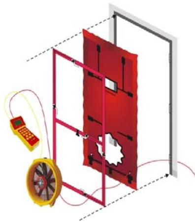
*Figure 2: The breakdown of a typical Blower Door fan system*
