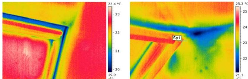
Figure 8: Connection of the roof window panel to the cladding before (left) and during (right) the blower door test
