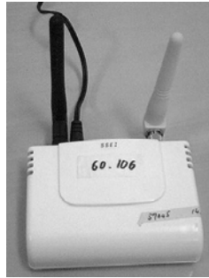
Figure 2. A repeater (The white pole is an antenna for IEEE802.15.4. The black pole is for IEEE802.11g)
