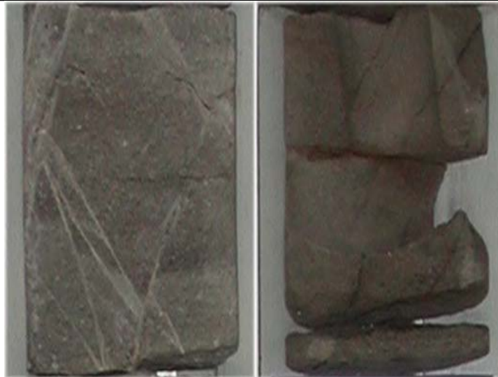
Figure 3: Examples of secondary mineralization cemented fractures (A-left, carbonate; B-right, pyrite)
