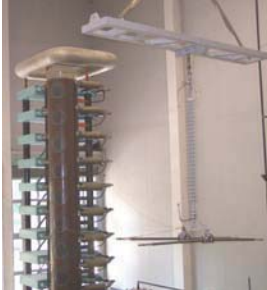
Fig. 2. A: 110 kV single suspension polymer insulator string
