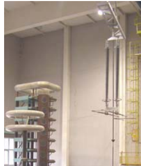
Fig. 5. D: 220 kV double suspension polymer insulator string
