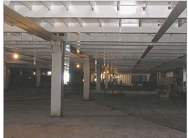
Fig. 1 Rectangular pillars supporting longitudinal girders of a car-deck on a car-carrier
