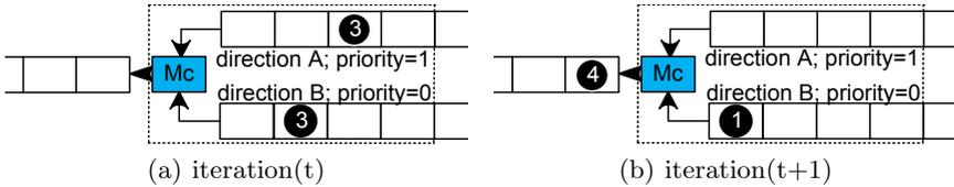
Fig. 4. Example of using the pass acceptance algorithm in a merge cell
