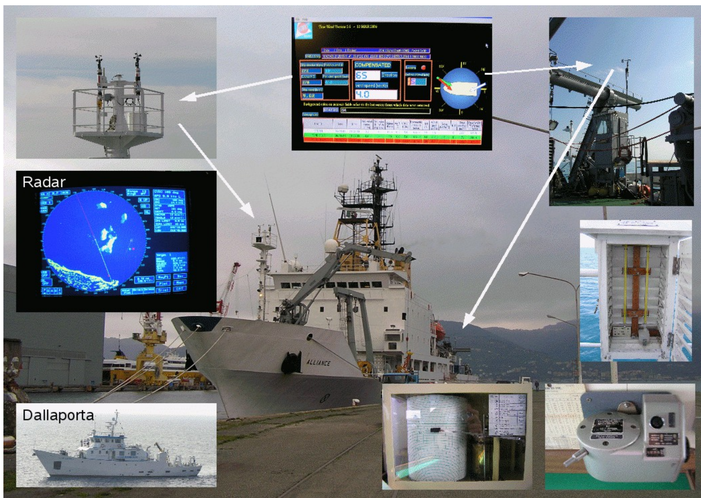
Figure 2: NRV Alliance at peer in La Spezia. The positions of automatic meteorological instruments are shown with arrows. Embedded figures show the meteorological instruments, computer interface for the measurements, ship's radar echo of a cloud and Dallaporta ship involved in the experiment.
