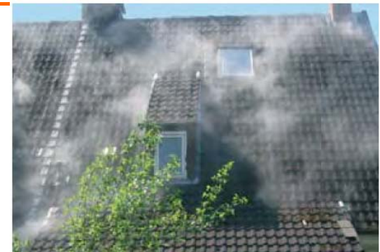
Smoke pressed out by a Blower Door fan to show the roof leaks
