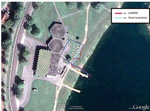
Fig. 9. GPS testing – output frequency 10Hz – clear view to the sky
