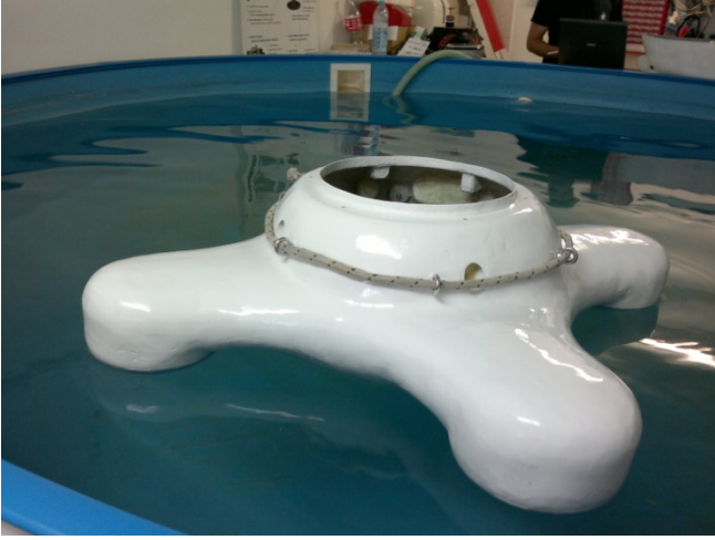
Fig. 2. Platform for dynamic positioning constructed in LABUST
