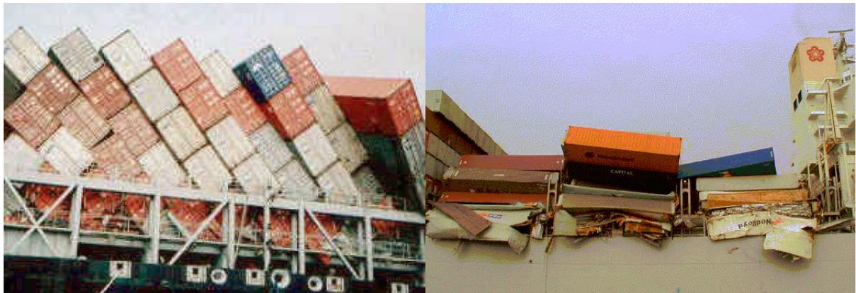
Figure 1-1. Casualties due to the parametric rolling on APL China.
