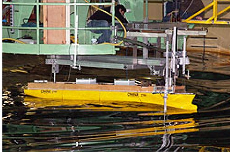
Figure 6-3. Experimental setup for the parametric rolling tests
