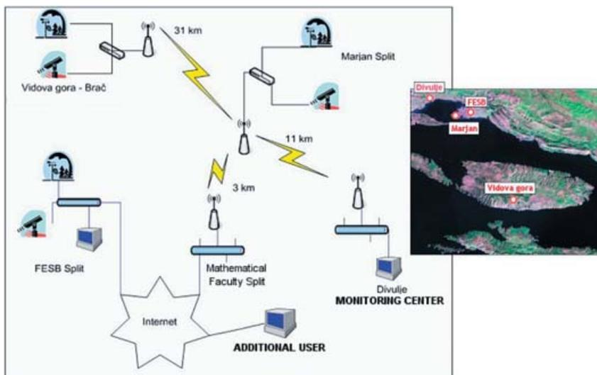
Figure 9 – The experimental system layout used for iForestFire prototype testing in 2004 and 2005
