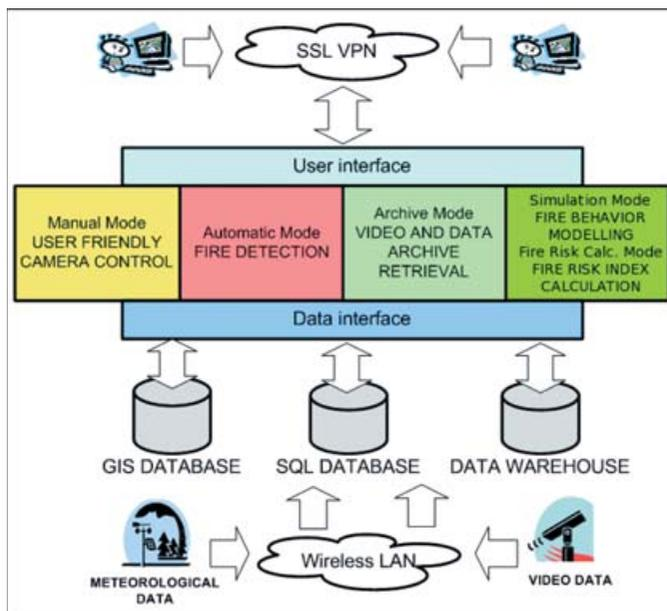
Figure 4 – The structure of iForestFire system
