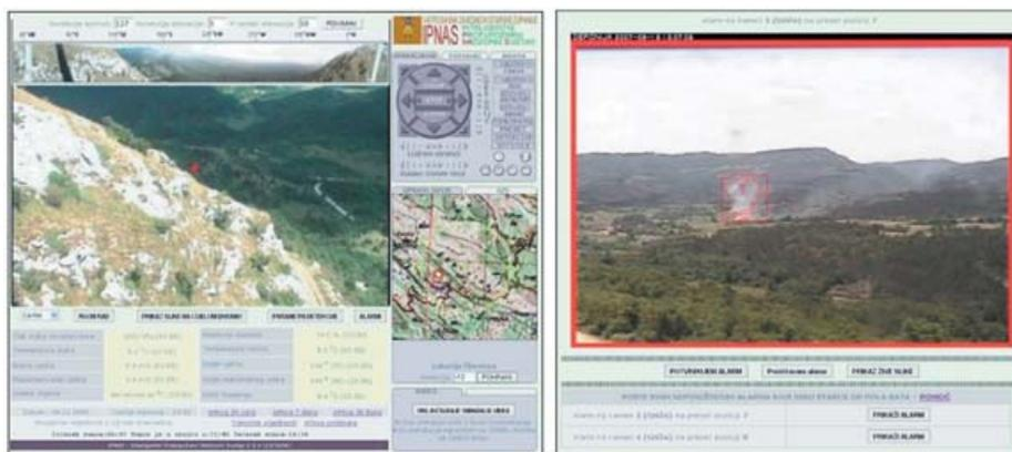
Figure 5 - iForestFire camera control screen with various manual control modes and typical fire alarm screen at location Buzet in Istria. The user can accept or discard the generated alarm.
