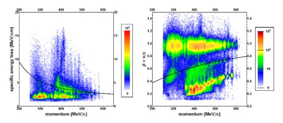
**Figure 1.** Identification of positively charged particles by their specific energy-loss (left) and their relative velocity (right) in the momentum range of the KAOS spectrometer. The expectation for kaons is indicated by the solid lines. Pre-selection cuts have been applied to suppress the background of positrons and pions (found at  $dE/dx \approx 2-3$  MeV/cm and  $\beta \approx 1$ ), and of protons (found at  $\beta \approx 0.2-0.4$ ).
