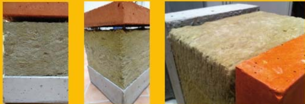
Image 1: ECO-SANDWICH is recycled concrete sandwich facade panel. Section detail and details in a perspective view.
