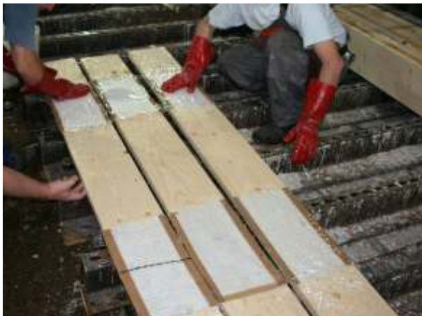
Fig. 1 Reinforcing gluelam timber specimens
