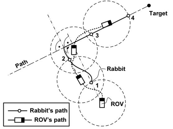
Fig. 2. Positioning of a dynamic virtual target (rabbit), relative to the ROV
