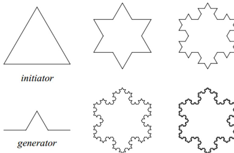
Figure 1.10: Generation of a snowflake
