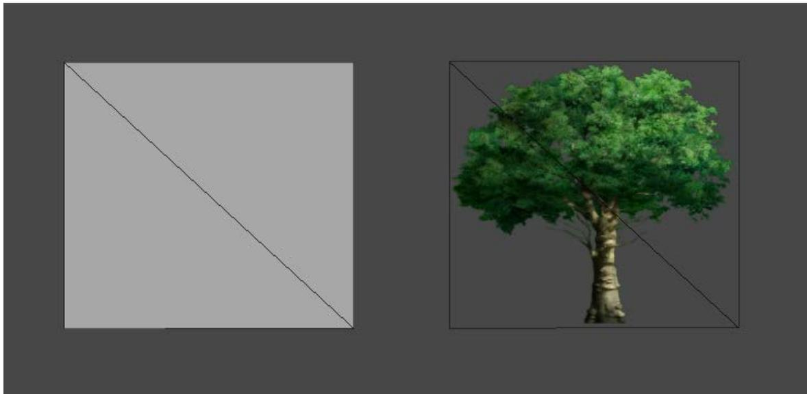
Figure 1.2: Left – a simple billboard consisting of two triangles, Right – same billboard but with a transparent texture applied
