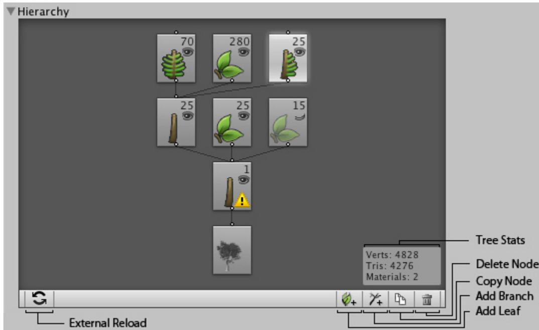
Figure 3.1: This hierarchy represents a tree with one trunk, 25 child branches. Child branches have in total 70 fronds attached, 280 leaves and 25 fronds with branches.
