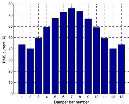
Fig. 12 No-load, RMS currents in the damper winding bars, delta connection
