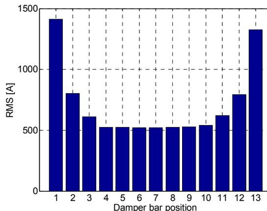
Fig. 4 Damper bar current distribution of one salient pole, two-phase load 1.5 MVA, delta connection
