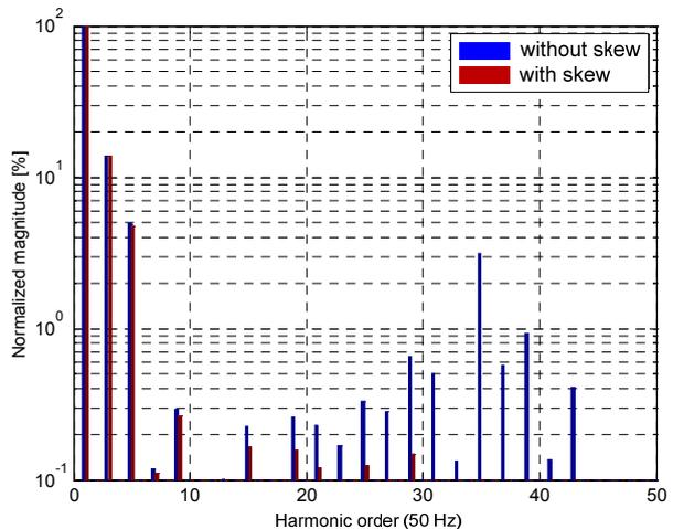
Fig. 11 Single phase load 1.5 MVA, line-to-line voltage, frequency spectrum, wye connection
