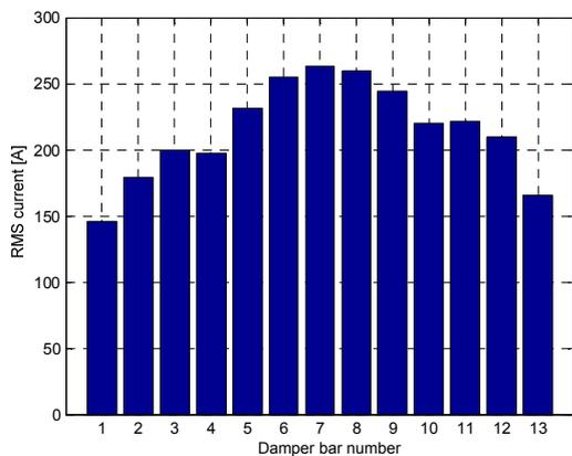
Fig. 13 Rated load, RMS currents in the damper winding bars, delta connection
