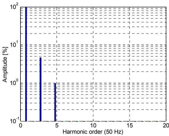
Fig. 7 Phase current frequency spectrum, two-phase load 1.5 MVA, wye connection
