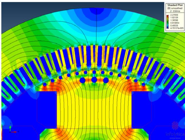
Fig. 3 Magnetic flux of a synchronous generator at unsymmetrical load
