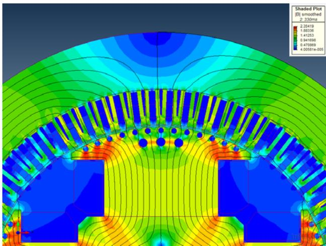
Fig. 2 Magnetic flux of a synchronous generator at rated load
