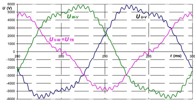
Fig. 9 Line-to-line voltage waveform, two-phase load 1.5 MVA, wye connection
