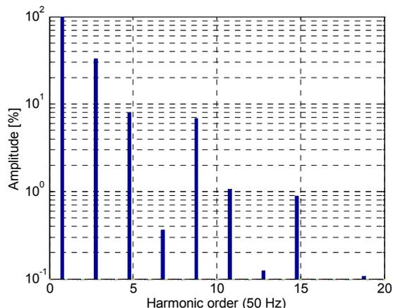
Fig. 6 Phase current frequency spectrum, two-phase load 1.5 MVA, delta connection
