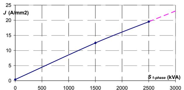
Fig. 14 Damper bar current as a function of two-phase load, delta connection
