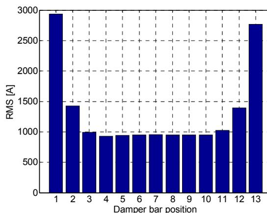
Fig. 5 Damper bar current distribution of one salient pole, two-phase load 1.5 MVA, wye connection
