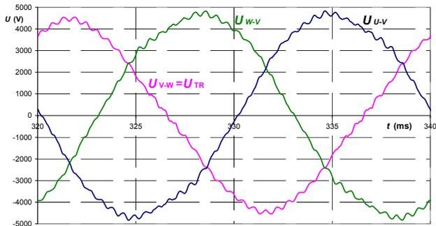
Fig. 8 Line-to-line voltage waveform, two-phase load 1.5 MVA, delta connection
