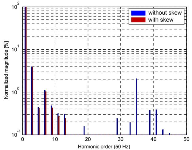
Fig. 10 Single phase load 1.5 MVA, line-to-line voltage, frequency spectrum, delta connection
