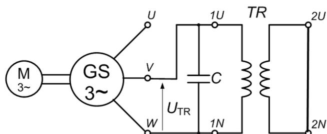
Fig. 1 Connection of a synchronous generator and a single-phase transformer during short-circuit test and the temperature rise test of the transformer
