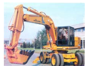
Figure 1. The physical model of an excavator: a - an undercarriage part; b - a revolving part; c - an arrow; d - an arm e - a bucket
