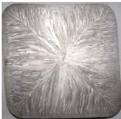
Fig.1. Macrostructures of sample 1 without Electromagnetic Stirring
