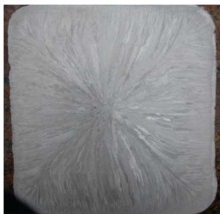
Fig. 2. Macrostructures of sample 2 under conditions of 5Hz and 320A
