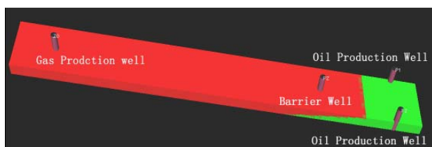
Fig.1 Schematic Chart of Numerical Model for Oil Reservoir
