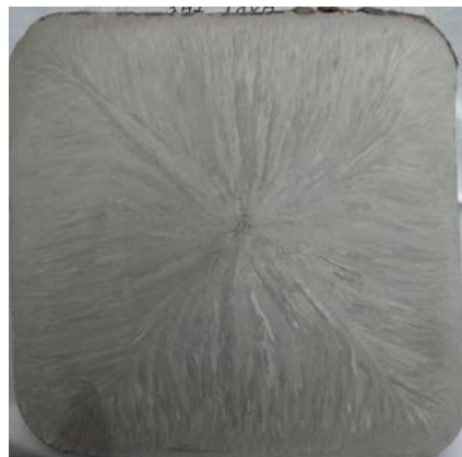
Fig.4. Macrostructures of sample 4 under conditions of 5Hz and 360A
