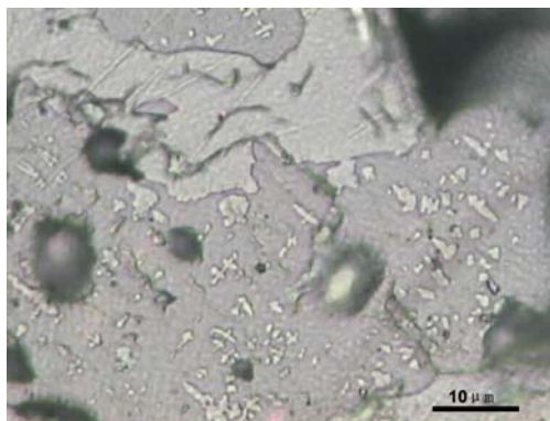
Fig. 2 Metallographic image of the (NiFe 2 O 4 -10NiO)-17(Cu-20Ni) cermet surface after electrolysis for 10 h
