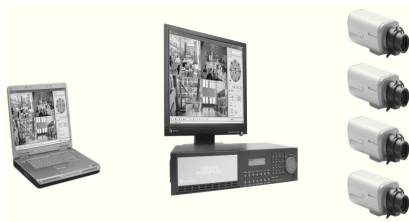
Figure 3 The elements of a modern system of digital video surveillance
