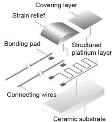
FIGURE 1. Design of a thin film sensor.
