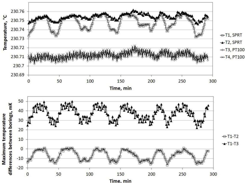
FIGURE 2. Stability and gradients in the MEFP when used as ordinary equalizing block, without phase transition.
