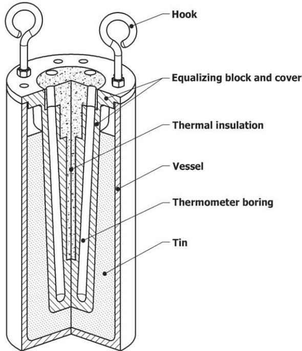
**FIGURE 1.** Schematic of the tin-filled Multi-Entrance Fixed Point.
