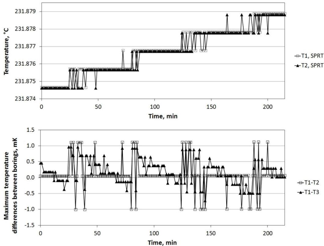
FIGURE 3. Stability and gradients in the MEFP during melting.
