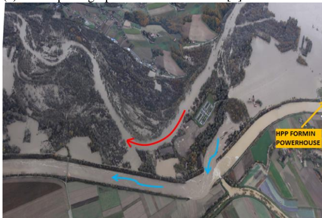
Fig. 7 Upstream levee breach of HPP Formin outlet canal
