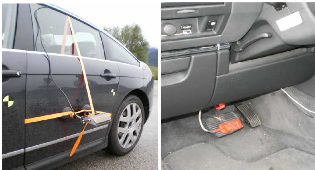
Figure 4 Attachment of microwave and brake sensor on the vehicle
