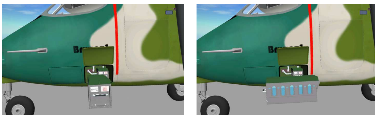
Figure 10 Checking of on-board rechargeable batteries and electrolyte level
