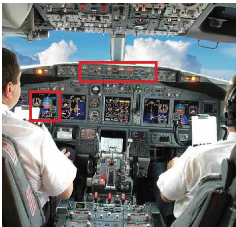
Figure 7 Aircraft cockpit; in rectangular marked pilot's AP/FP Mode Control Panel (detail in Figure 8) and pilot's primary flight display = FPD (detail in Figure 9) [5]
