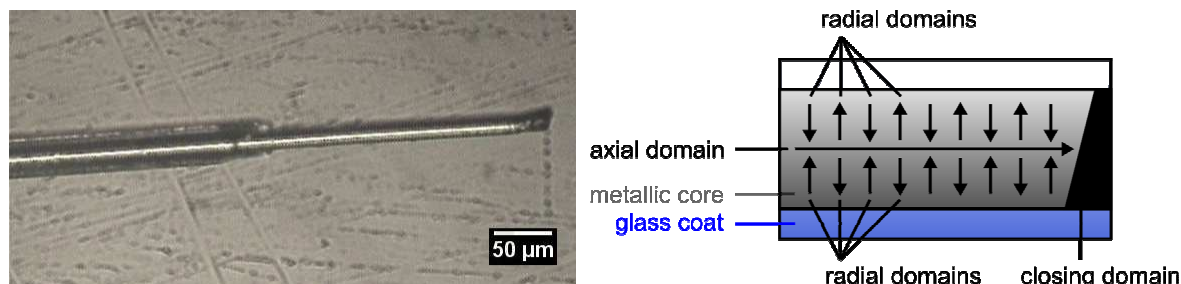
Figure 1 Amorphous magnetic microwire with high and positive magnetostriction constant and its domain structure schematics
