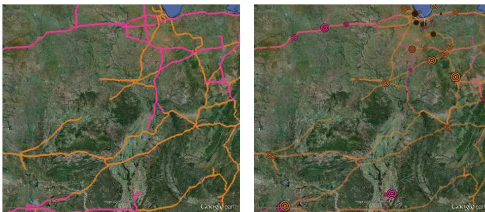
Figure 1 Two truck trajectories, marked magenta and orange respectively, are displayed with Google Earth. The trajectories of several thousand kilometres each are displayed in opaque (left) and in transparent (right) modes, respectively. The locations of abrupt braking events are marked in the right image.
