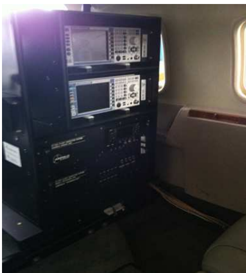
Figure 2 Airborne and ground equipment AT-940 with spectral analyser and selective millivolt meter.
