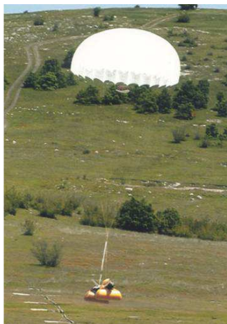
Figure 1 UAV parachute recovery system fitted with airbags [5]
