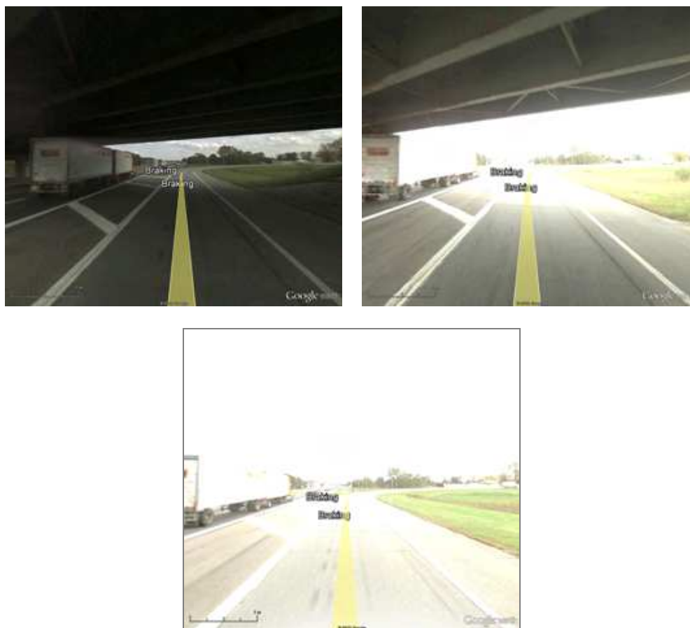
Figure 3 b - d: Frames with sudden change in illumination recorded by the panoramic camera mounted on Street View car near a truck braking location recorded in the trajectory and braking database at a different time.
