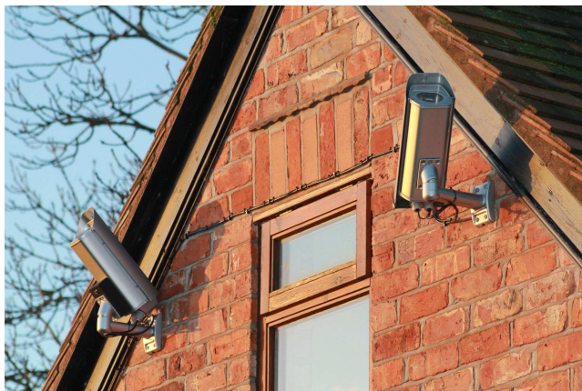
Figure 1 – Both cameras of the Ravensmoor Node permanently affixed to the gable end of a brick building. The unit on the left faces east while that on the right faces north. Note the black spacer block on the left hand unit between the camera housing and the mounting bracket. This modification was required in order to allow the appropriate elevation to be achieved without the rear of the housing fouling on the horizontal support bracket.
