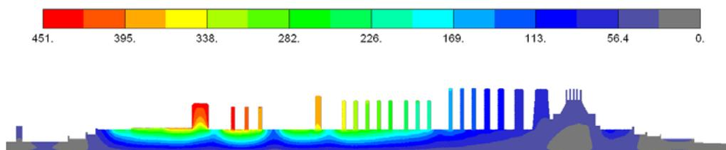
Figure 2. Temperature field ( $^{\circ}\text{C}$ ) in the rotor during cold start-up [3]
