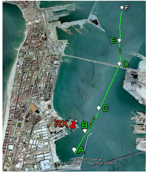
Fig. 2. Fixed location of the receiver antenna onshore (RX) and route followed by the ship (from A to F) during the measurement campaign.
