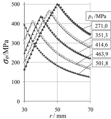
**Fig. 4.** Comparison of analytical and FEM results of circular stress distribution
