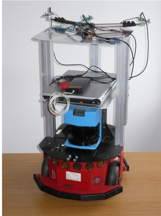
Figure 2.2: Mobile robot equipped with a four channel microphone array
