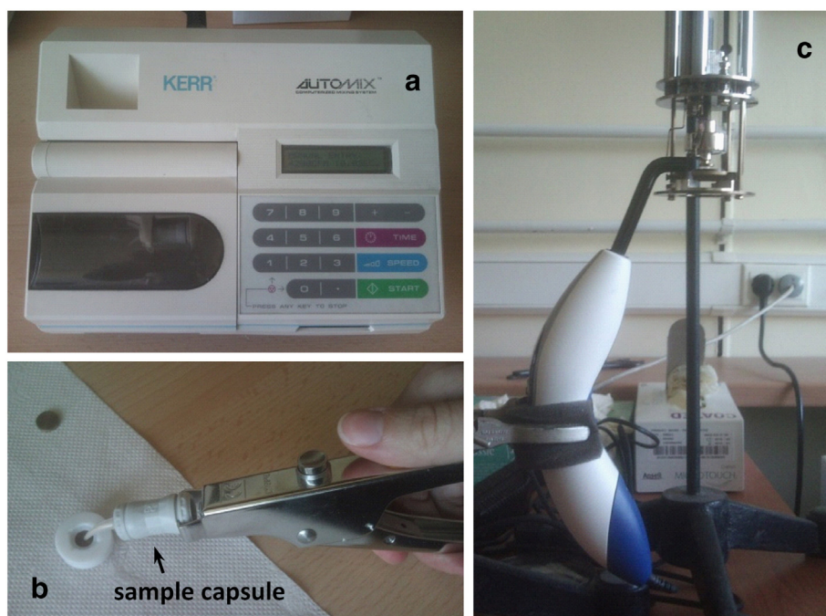
Fig. 1. Sample capsule, which contains glass powder and liquid, is first activated and placed into the AUTOMIX mixer to mix the two components (a); using an applicator the paste is extruded into the Teflon mold (b) or quartz ring; the sample in the mold/ring is placed in the impedance cell and activated by Bluephase lamp (c).
