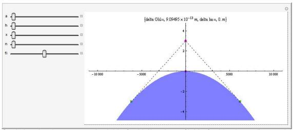
$G_{hi}$  – horizon along the curvature arc;  $h_a$  – height of aerial;  $\Delta h_a$  – change of height of aerial on the vessel's mast, relative to the sea level;  $\alpha$  – angle of rolling
