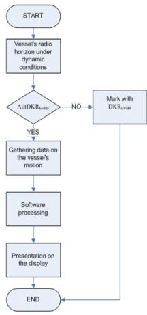
Figure 5 Algorithm for operation of the automated system (*AutDKR*<sub>hVHF</sub>) Slika 5 Algoritam rada automatiziranog sustava (*AutDKR*<sub>hVHF</sub>)
