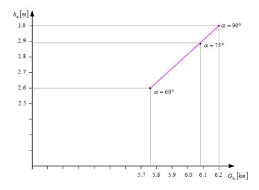
$G_{hl}$  – horizon along the curvature arc;  $h_a$  – height of aerial;  $\alpha$  – angle of rolling
