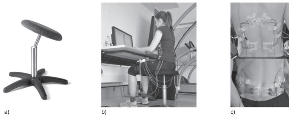
Figure 1: Representation of a) a novel chair with unstable seat (Active Chair<sup>®</sup>), b) a computerized office task while measuring EMG activity on the Active Chair<sup>®</sup> and c) EMG electrodes positions for left and right lower trapezius and erector spinae (upper picture) and rectus abdominis and obliquus externus (lower picture) muscles.
