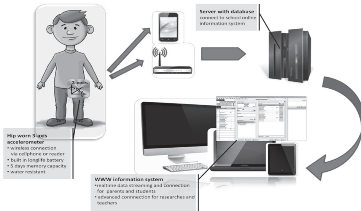
Figure 1: Algorithm of data recording, transfer and evaluation
