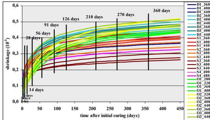
Figure 1: Concrete shrinkage test results for all compositions (specimens cured in water for two days) presented via shrinkage approximation curves
