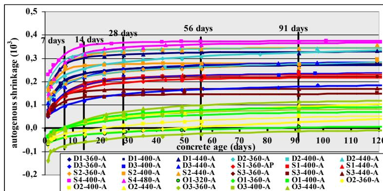
Figure 2: Autogenous shrinkage test results (measured values rather than corrected values are given for groups O1 and O2)
