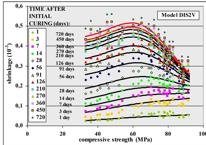
Figure 4: Relationship between shrinkage and compressive strength in different time intervals after the end of initial cure of concrete, with shrinkage approximation curves based on the DIS2V model
