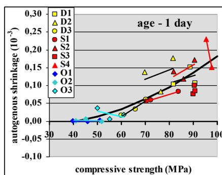
Figure 3: Autogenous shrinkage of concrete corrected for deformation due to change in temperature and negative shrinkage approximated by parabola
