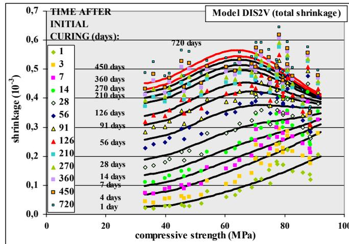
Figure 5: Shrinkage approximation curves according to the total-shrinkage experimental model DIS2V
