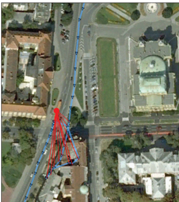
Figure 2b Recorded GPS track and actual PT vehicle position, (Jelušić et al., 2010)
